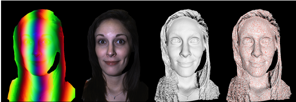
Fig. 6.3. Encoding and decoding 3D geometry and color texture. A lossless PNG format results in a compression ratio of approximately 112:1. Images from left to right respectively show the encoded RGB PNG image, the recovered color texture, the 3D reconstructed geometry, and an overlay of the reconstructed 3D geometry on top of the original 3D geometry (gray color represents recovered geometry and red represents the original geometry).
