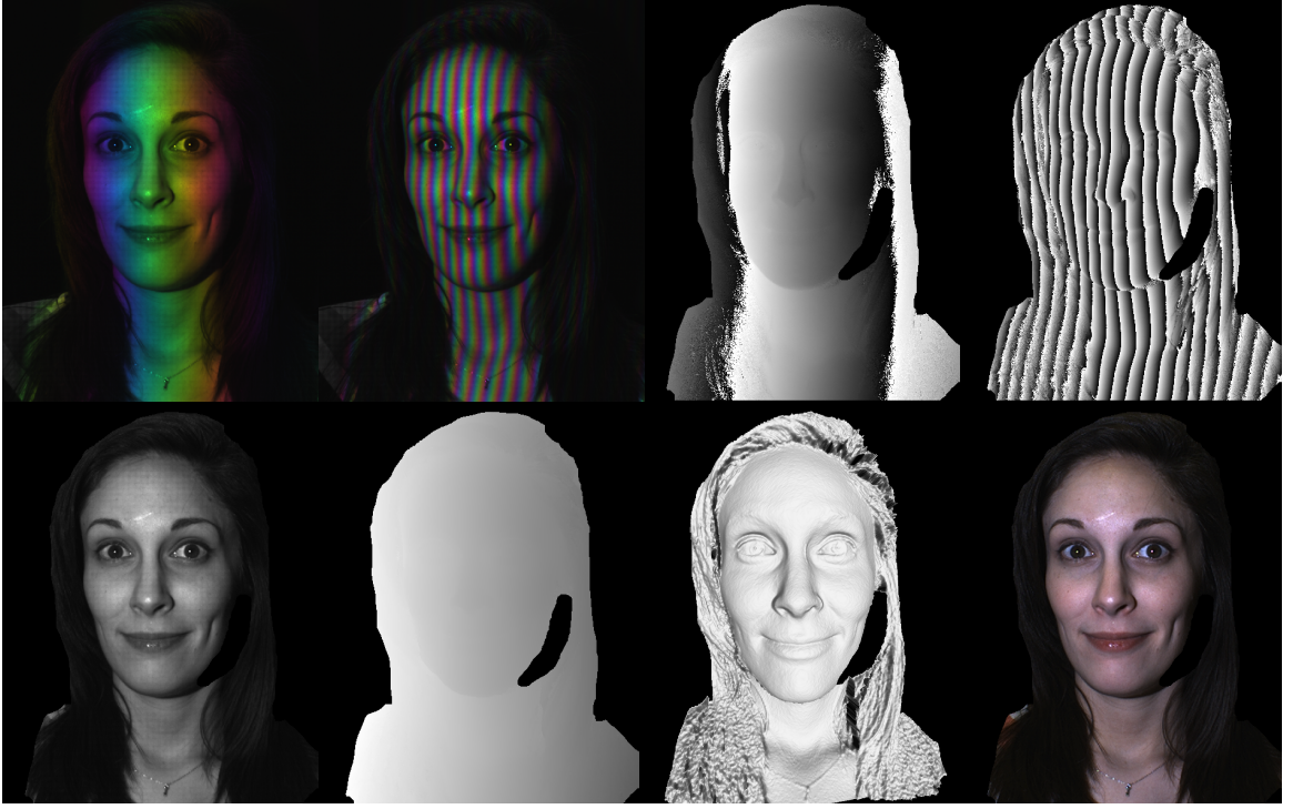
Fig. 6.2. Example of reconstructing 3D geometry and color texture from the Acquisition Module. Top row left to right: low frequency fringe patterns, high-frequency fringe patterns, low frequency wrapped phase \phi^l , high-frequency wrapped phase \phi^h ; bottom row left to right: b/w texture I_t^g , unwrapped phase \Phi , 3D geometry, color texture after demosaicing I_t^c .
