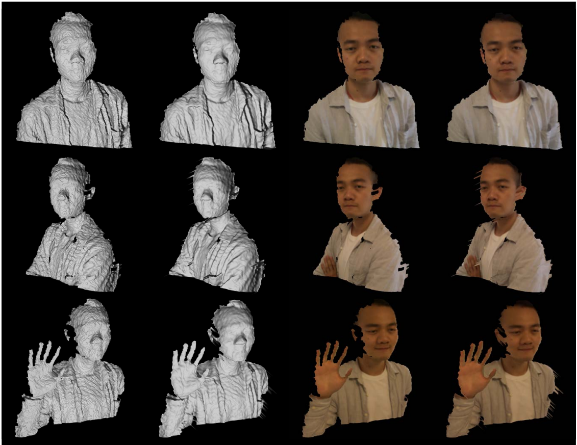
Fig. 6.11. The Mobile Holostream platform was used to capture, compress, and transmit 3D video of a dynamic scene representing a 3D video conference. Each row shows reconstructions of the individual at different times. Column one: lossless reconstruction of the 3D data as captured by the sending iPad; column two: 3D data reconstructed from lossy H.264 video received by the receiving iPad; column three: lossless reconstruction of the 3D data as captured by the sending iPad with color texture mapping; column four: 3D data reconstructed from lossy H.264 video with color texture mapping.
