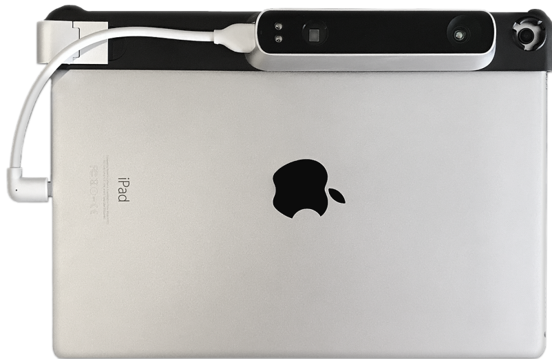
Fig. 6.7. The Structure Sensor (Occipital, Inc.) attached to an iPad Pro. The Structure can provides the iPad with 640 \times 480 depth maps at 30 Hz. In addition, the iPad's color camera can be used to provide color texture information.
