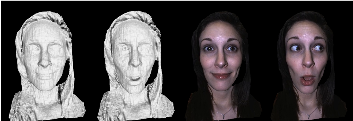
Fig. 6.6. Compressing encoded 3D data with the H.264 video codec at very lossy (CRF of 25) qualities achieving a 16,279:1 compression ratio.
