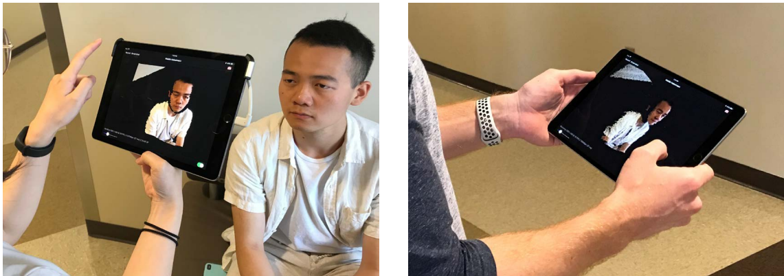
Fig. 6.8. The Mobile Holostream platform in use. The left image shows the Mobile Holostream platform that uses an iPad Pro and a Structure Sensor to capture, compress, and wirelessly deliver 3D video data of a person in real-time. The right image shows another person using the Mobile Holostream platform on another iPad to receive, decompress, visualize, and interact with the reconstructed 3D video data in real-time.
