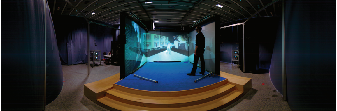
Fig. 2.5. The blue-c telepresence portal [13]. Three large projection screens and projectors outside of the screen are used to display a virtual environment to the user. The cameras positioned on the metal scaffolding outside the system are used to capture the geometry of the user within which will be transmitted for display within a remote blue-c node.
