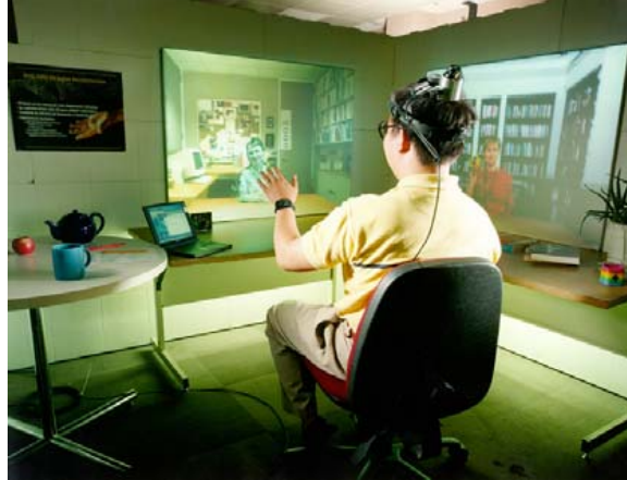
Fig. 2.4. A user sits in front of the system developed by Towles et al. [12] for remote 3D tele-collaboration. The system uses an array of cameras to capture a colored 3D point cloud of the user which is then transmitted across a network to remote participants.
