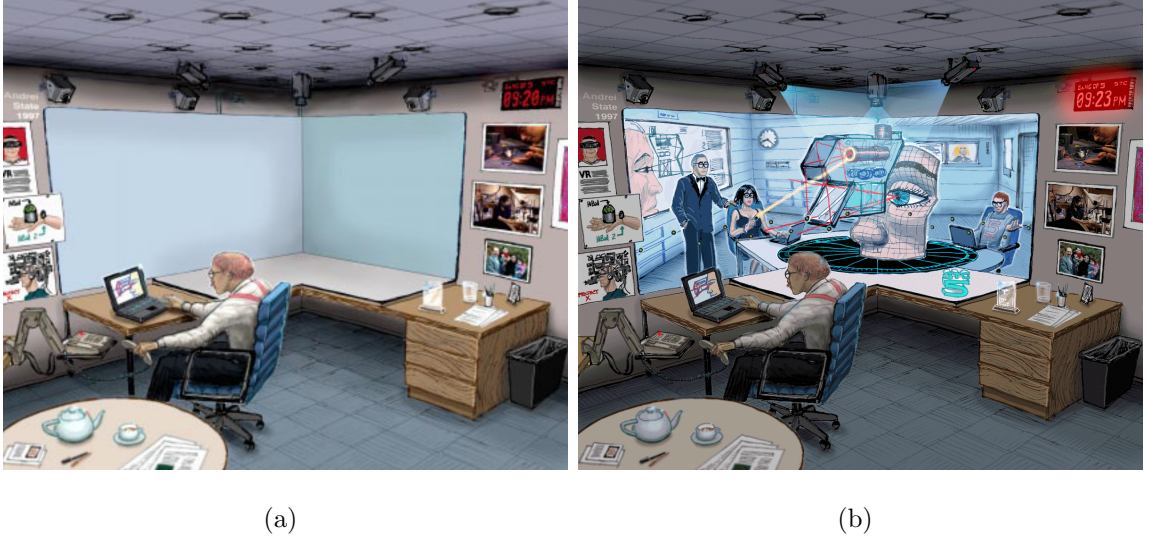
Fig. 2.3. A sketch of the proposed office of the future [11]. (a) Cameras and projectors on the ceiling and walls of the office 3D scan the user, their workplace, and the objects within; (b) the projectors turn the walls into a virtual collaborative working environment by projecting the 3D scans of other users, their offices, and objects into the user's physical space.
