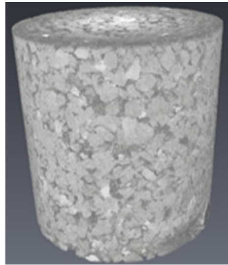
Fig. 12. Gray image of a cylindrical core imaged by micro-CT.
