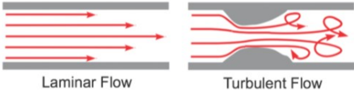
Figure 1.3. Blood flowing through a healthy artery and a stenosed artery – The flow regime shown in a healthy artery that contains Laminar Flow; the stenosed artery on the right contains turbulent flow. IMAGE: [14]
