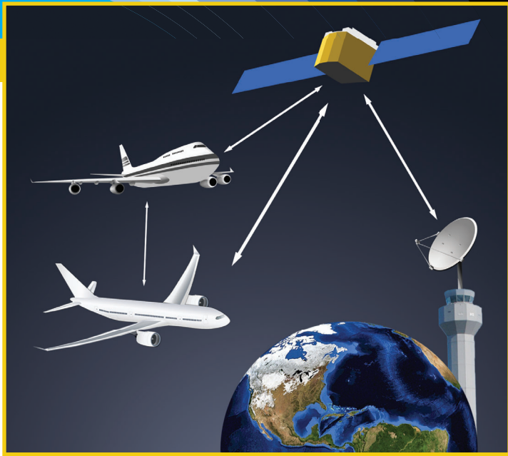
Figure 1: How space-based ADS-B works
