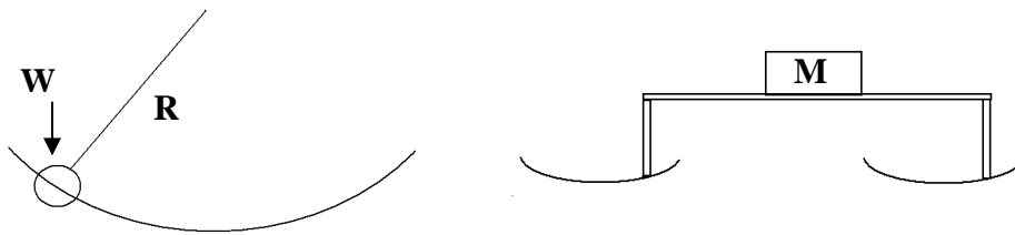
Figure 3. Concept of sliding pendulum motion 1
