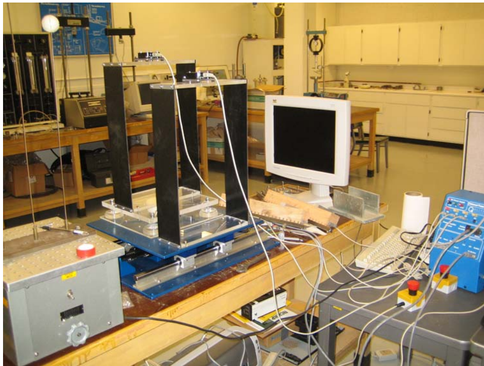
Figure 7. Experimental setup on shake table
