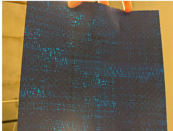
Figure 5.13. Carbon fiber prepreg held to the light to show general fiber misalignment and gaps.
