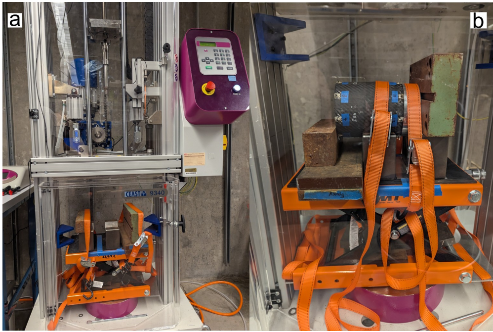
Figure 5.9. a) CEAAT impact drop tower, b) SA specimen loaded into test frame with fixturing.
