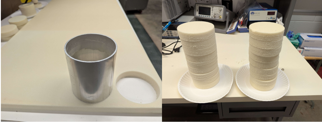
Figure 4.5. Al6061-T6 die cutting tool and resulting PIR foam mold pieces
