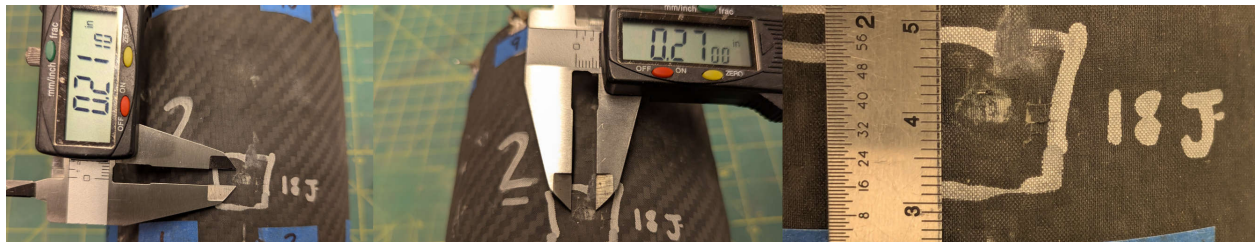
Figure 6.4. Location and sizing of 18 (J) impact damage in shell, dimensions in (in.).
