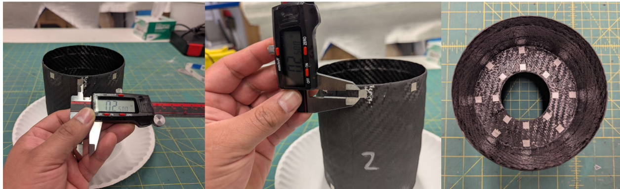
Figure 4.10. Electrode dimension measurements for shell: length and width and annulus electrodes.
