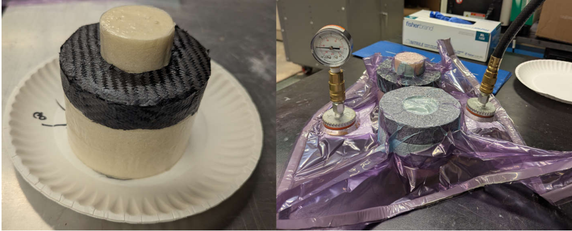
Figure 4.7. CFRP annulus laminate halves layup under debulk.
