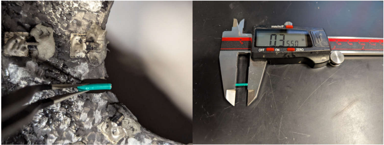
Figure 6.2. Annulus after cutting of the notch with the length verification.
