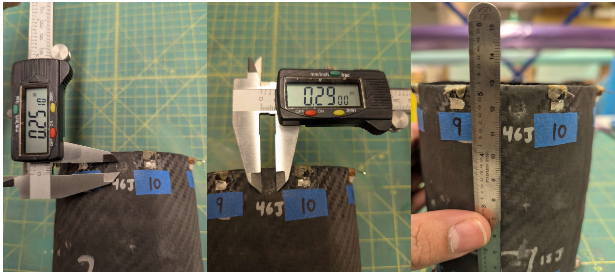
Figure 6.6. Location and sizing of 46 (J) impact damage in shell, dimensions in (in.).
