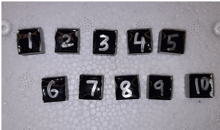
Figure 3.2. Representative DC specimens. The left and right side faces have fast drying silver paint to form surface electrodes.
