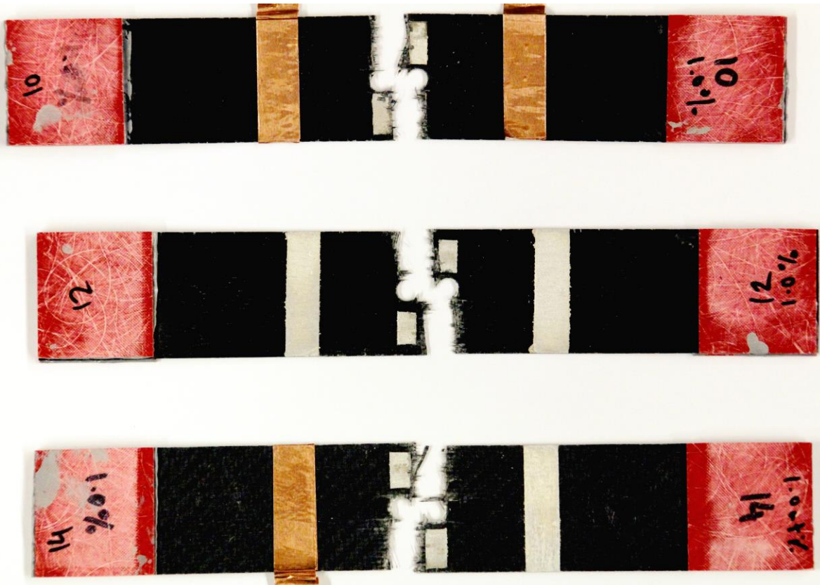
Figure 5.3: GFRC with CNF-modified epoxy added at 1.0 wt.%. Sample 1, 2, and 3 are labeled 10, 12, and 14 respectively.
