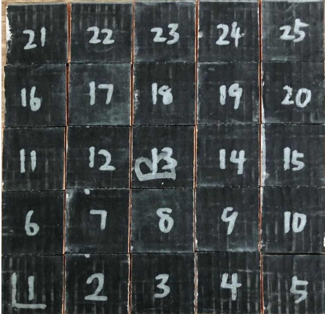
Figure 4.1. 25 0.5 wt.% CNF-modified glass fiber/epoxy 1" × 1" inch square specimens used in AC conductivity measurements.
