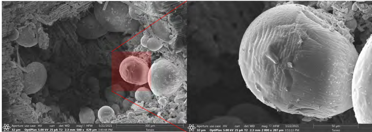
(b) Bubble formation within an ablation crater formed by a 20-second exposure on 1.0 wt.% CNF-modified GFRC specimen as seen at 500 \times magnification. The magnified image (at 2000 \times magnification) shows topography of a bubble.
