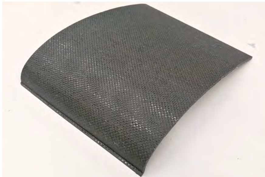
Figure 4.3. A cured airfoil specimen used for testing. This airfoil is 4” in width with a chord length of 5.”
