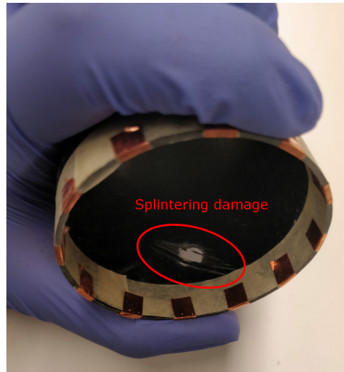
Figure 5.4: Occurrence of splintering damage. Splintering damage occurred because the holes were drilled without any backup
