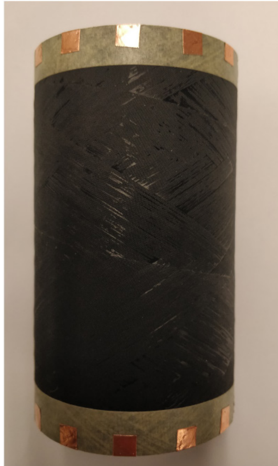
Figure 5.1: Specimen of length-to-diameter ratio 2:1 prepared for EIT. The copper electrodes are attached over a layer of masking tape to prevent current being injected through the sides. This ensures good correspondence with the forward model.
