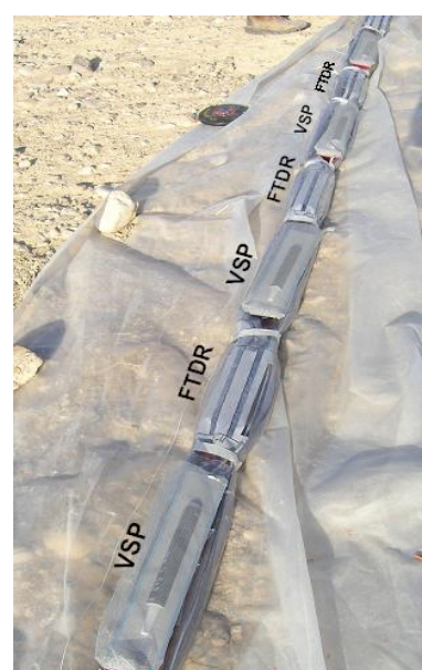
Figure 3: VSP and FTDR probes on flexible sleeves
