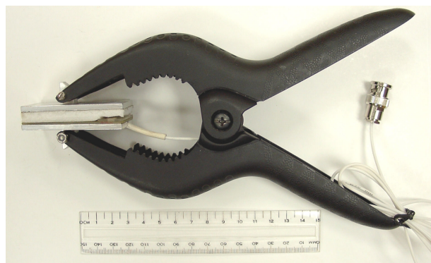
Figure 9b. Spring loaded clamp housing the circuit board TX line.
