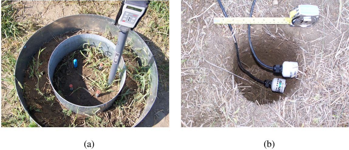
Fig. 3. (a) Double-ring infiltrometer with TDR probe (blue cap), Theta Probe, and tensiometers (red caps) and (b) Hydra Probes at 5 and 20 cm depths during installation.
