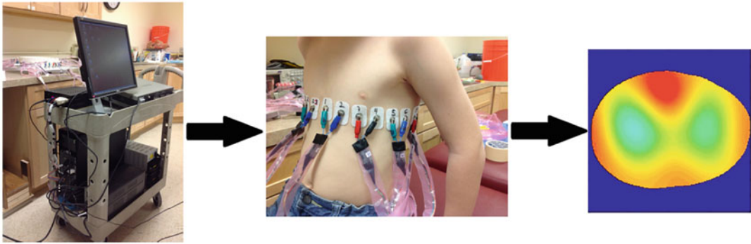
Fig. 1 Left: The ACE 1 EIT system on a cart in the lab at Colorado State University. Center: Electrodes on a healthy 8-year-old subject. Right: Example of an EIT image of the chest during ventilation. Regions of high conductivity are shown in red, and low conductivity regions in blue. The heart is at the top of the image and appears red; the lungs are blue
