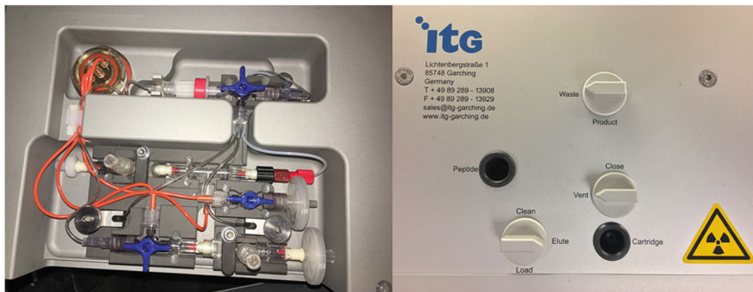
Fig. 10 Left: Plumbing system of the ITG iQS Fluidic Module , attached to the ^{62}\text{Cu} generator outlet and ready for ^{62}\text{Cu} -radiotracer synthesis. Right: Upon closing the lid, the stopcock valves are firmly engaged by the knobs visible on the top of the lid, allowing user control of the fluid pathways required in various stages of synthesis. External Luer fittings are accessible via the “Peptide” and “Cartridge” ports for reagent additions, as well as for pressurization to effect required fluid transfers
