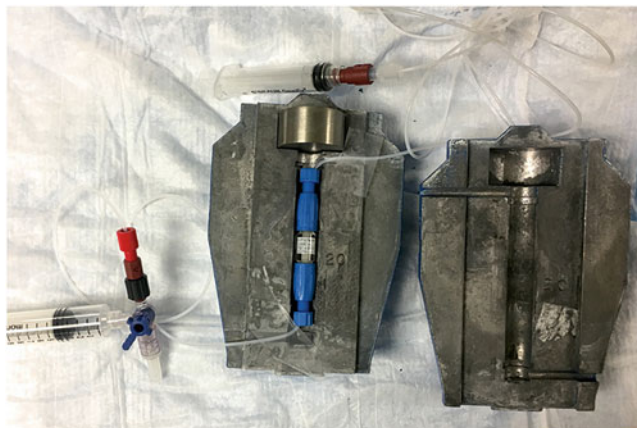
Fig. 8 Glass column containing Dowex 1 × 8 anion exchange resin (200–400 mesh) positioned in lead shielding in preparation for loading with the aqueous HCl solution of ^{62}\text{ZnCl}_4^{2-}
