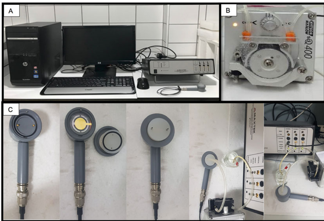
Fig. 4 (a) Quartz crystal microbalance (QCM) apparatus, (b) Peristaltic pump, and (c) Schematic of QCM sensor system preparation
