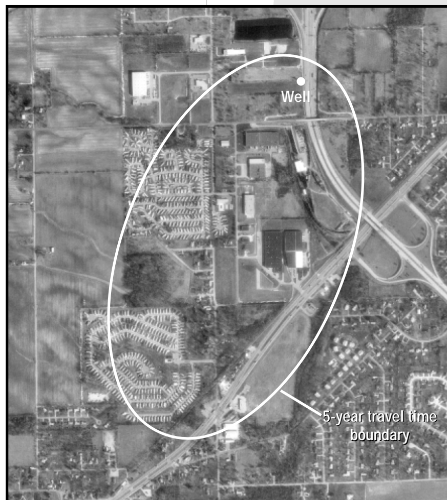
Figure 1. A wellhead protection area ideally encompasses the area from which ground water can travel to the well in five years or less. The wellhead protection area is elongated because of normal ground water flow.
