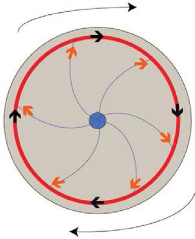
Fig. 8. Paths followed by the reactant gases above the susceptor.
