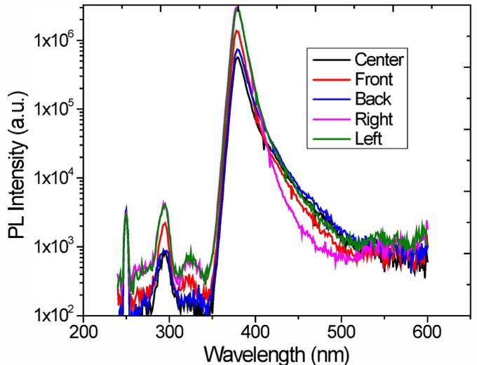
Fig. 4. Photoluminescence spectra at five different points for a sample grown at 600 °C.
