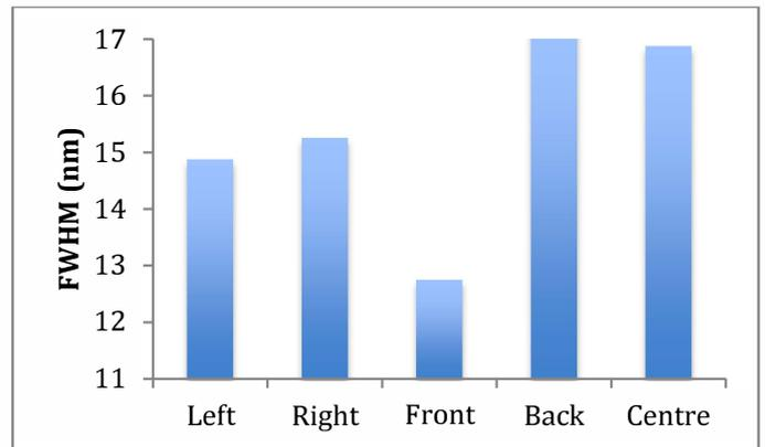
Fig. 3. Full width at half-maximum of the PL spectra at each of 5 points measured at room temperature.
