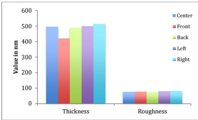
Fig. 5. Values of thickness and root mean square roughness as obtained by spectral reflectance by spatial positioning.
