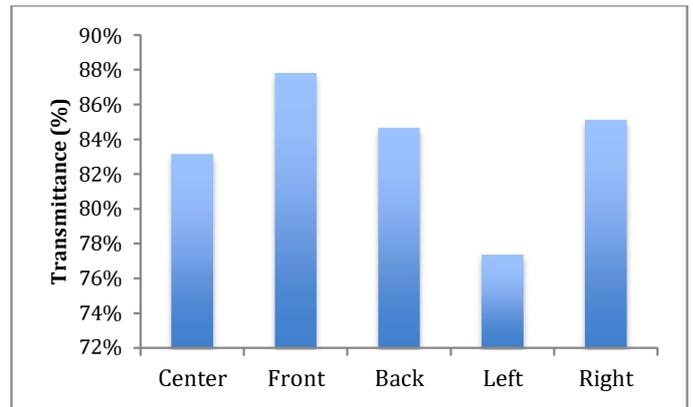
Fig. 7. Average transmittance values from wavelengths 390 nm to 1100 nm.
