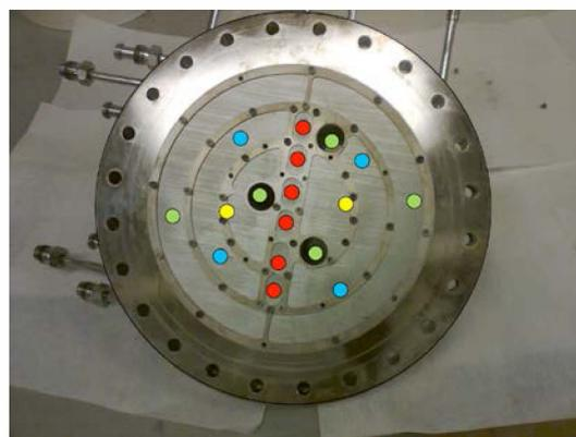
Fig 1. Flow flange for gas entrance into chamber. Red dots show DEZn entry points, blue for oxygen, green for nitrogen, and yellow for trimethylgallium for doping (not used).
