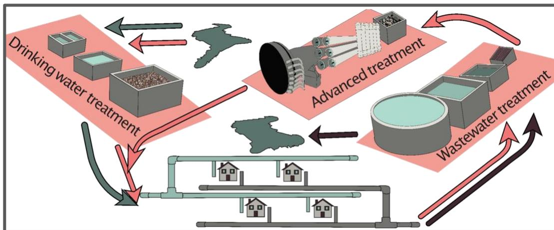
**Figure 1:** A simplified depiction of the engineered water cycle, where a drinking water distribution system conveys potable water to and a sewer system removes wastewater from residences. This depiction includes two surface water bodies, drinking water treatment (blue/green arrows), wastewater treatment (brown arrows), and direct potable reuse (pink arrows).
