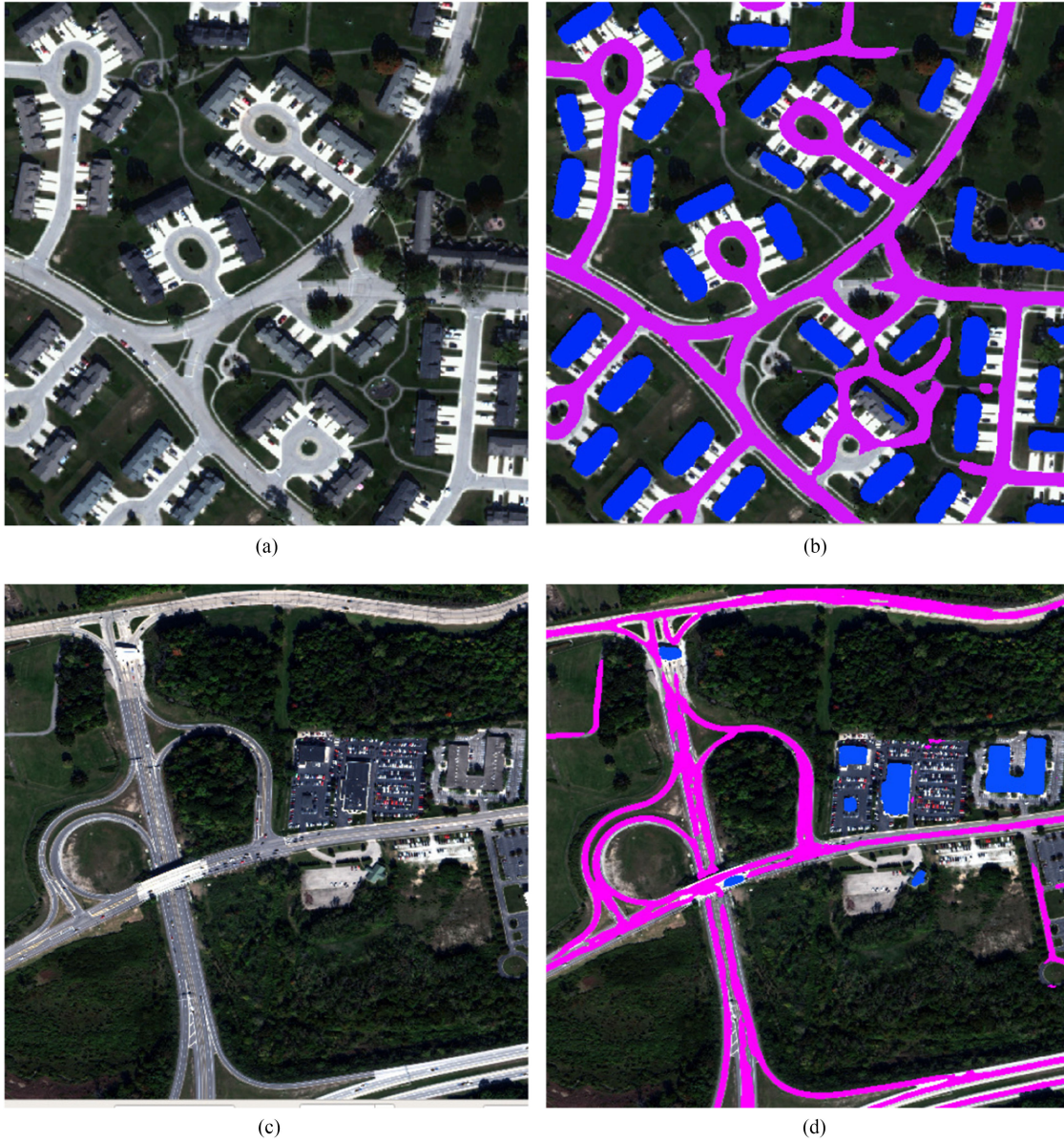
Fig. 6. Examples of orthorectified images and semantic labels output by our pipeline. Buildings are marked in blue and roads are marked in magenta. a) Ortho view. b) Predicted labels. c) Ortho view. d) Predicted labels.
