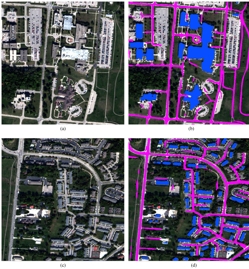
Fig. 8. Examples of orthorectified images and semantic labels output by our pipeline. Buildings are marked in blue and roads are marked in magenta. a) Ortho view. b) Predicted labels. c) Ortho view. d) Predicted labels.
