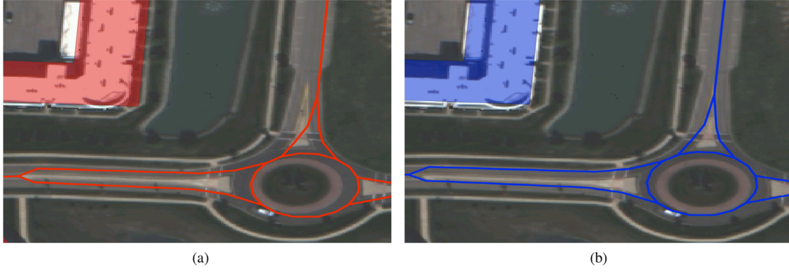
Fig. 12. Typical results obtained by aligning the orthorectified images with OSM. (12a) Unaligned OSM vectors overlaid (in red color) on top of an orthorectified image window. (12b) Aligned OSM vectors overlaid (in blue color) on top of an orthorectified image window.
