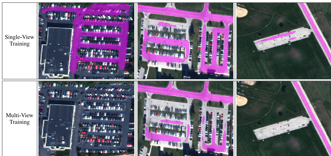
Fig. 9. Examples illustrating how multiview training helps to distinguish parking lots from true roads. Predicted road labels are marked in magenta.
