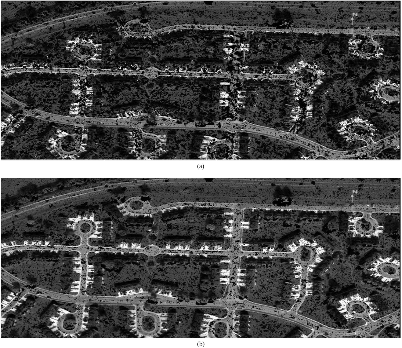
Fig. 10. Example to show why one cannot use a constant bias correction for a full-sized image. a) Ortho view of a portion of a pairwise point cloud constructed with the constant bias assumption. b) Ortho view of a portion of a pairwise point cloud constructed with tile-based bias corrections. The points have been colored using the color from the images.
