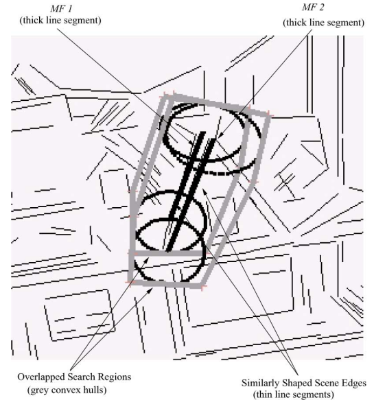
Fig. 7. Search regions for two different model lines overlapping significantly. Note that the search region for a model line is the convex hull of the two projected uncertainty regions for the two line extremities.
