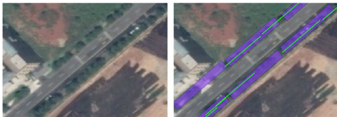
Fig. 13. Left: reference region with linear trees. Right: round truth rectangles are shown in purple and detections are shown as green lines.
