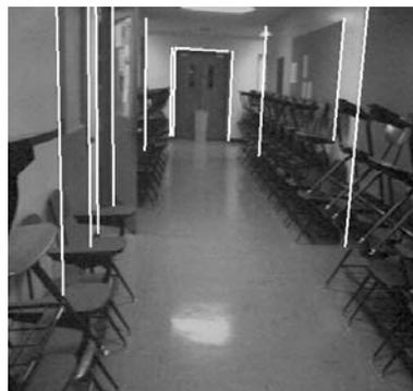
Figure 7: *Matched model features are projected back into the camera image. For this projection process, we use the estimated mean position of the robot to demonstrate the accuracy of the position estimation.*
