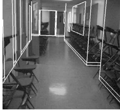
Figure 4: *A camera image taken for self-location. The white lines superimposed here indicate a scene expectation map rendered from a 3D model of the hallway.*
