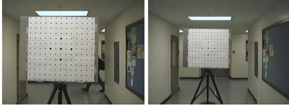
Figure 4: Images of the calibration pattern for automatic detection of landmarks used in Test Method 2
