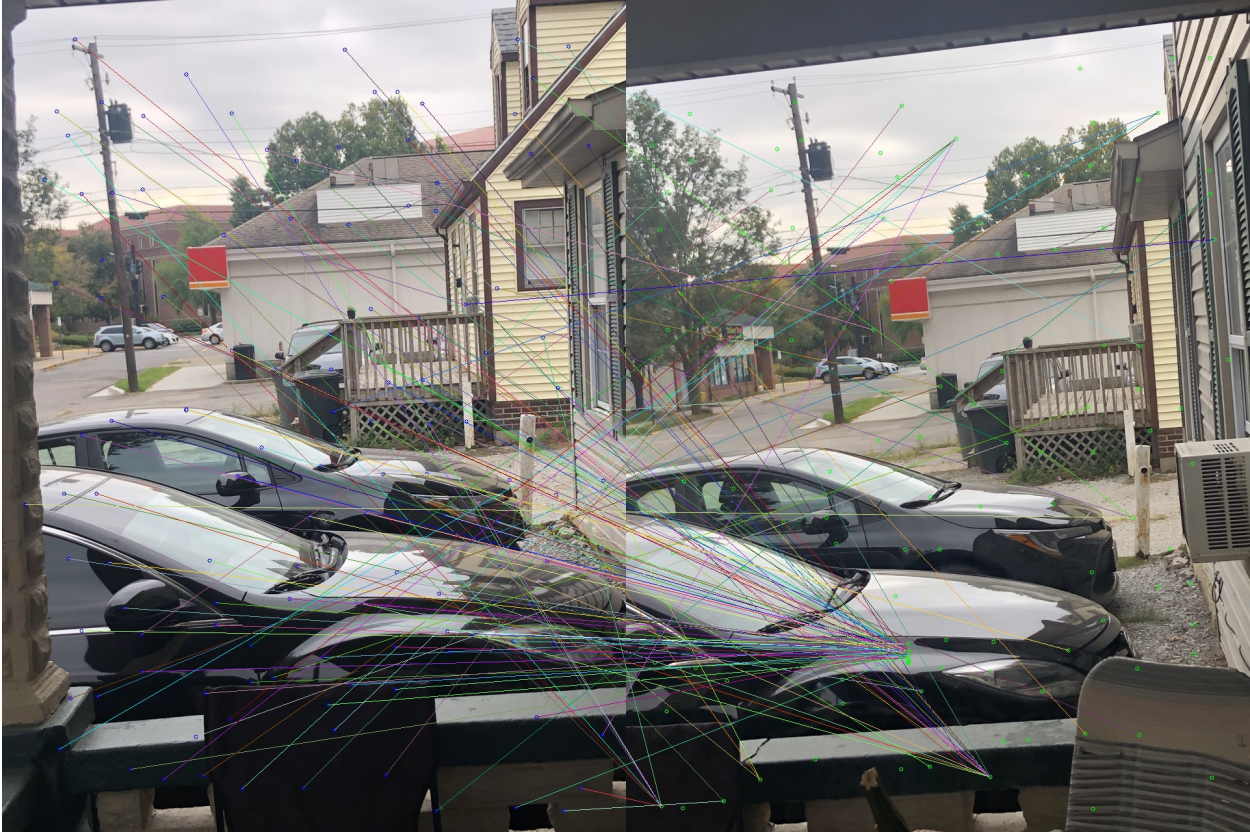
Figure 45: cars correspondences at \sigma = 13 using NCC
