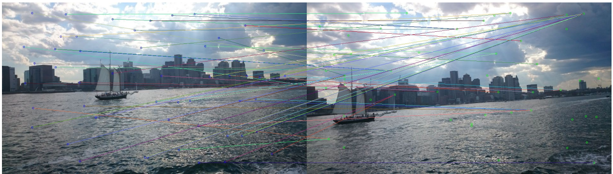
Figure 8: pair1 correspondences at \sigma = 13 using SSD
