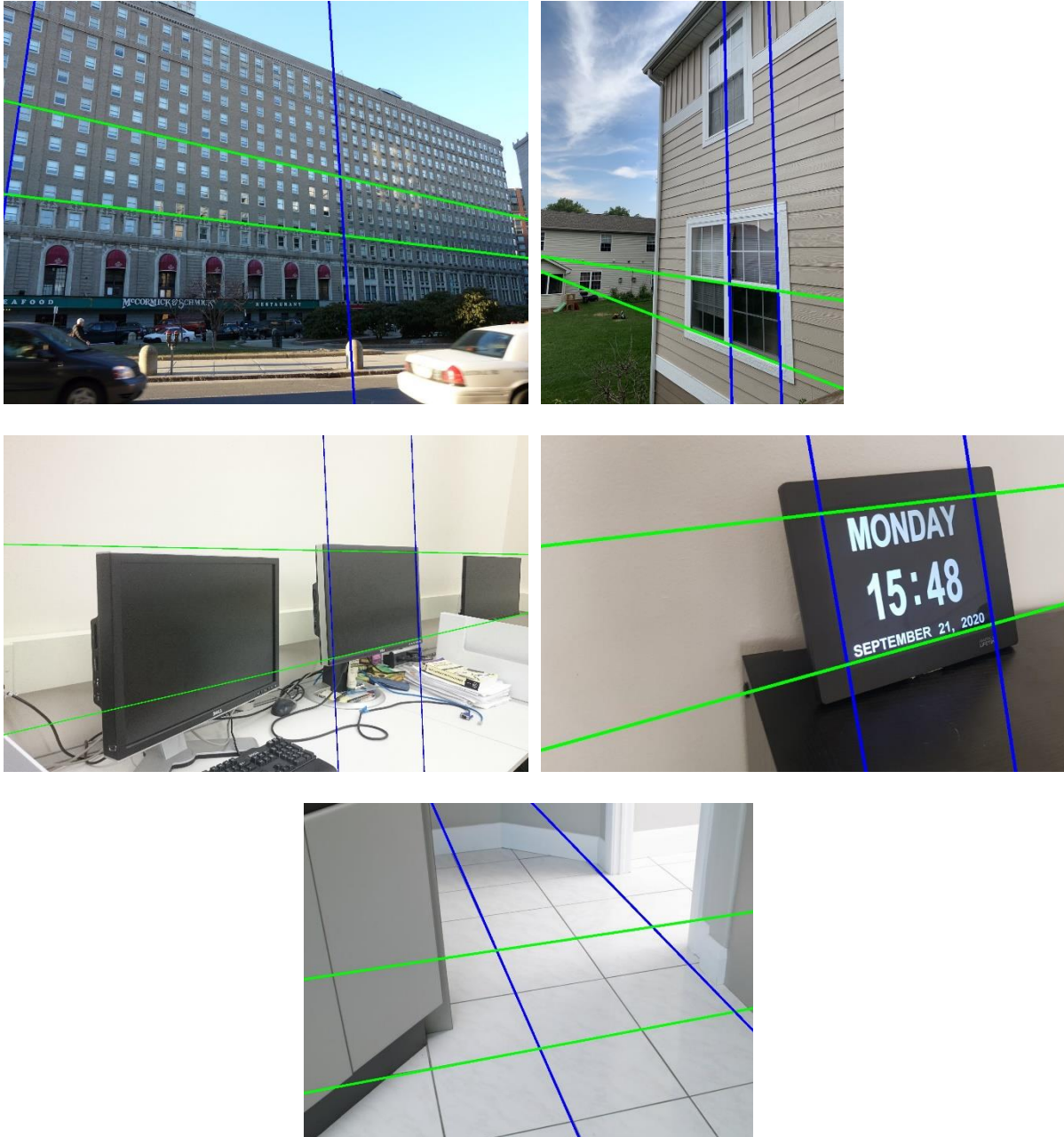
Figure 8: The parallel lines used to obtain the vanishing lines for Img1 (top left), Img2 (top right), Img3 (middle left), Img5 (middle right) and Img4 (bottom)
