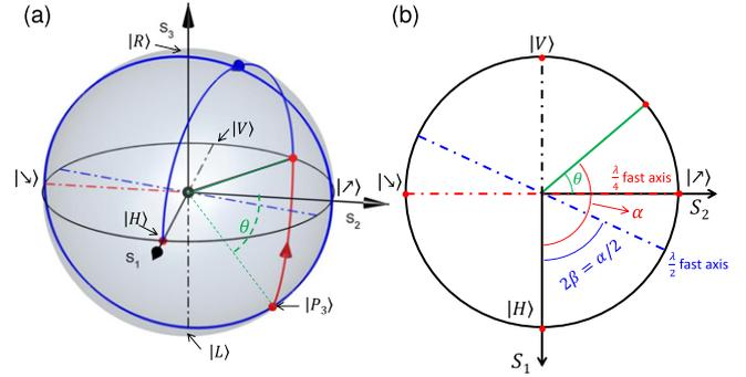
**Figure 2.** (a) The Poincaré sphere. An arbitrary projection state can be rotated to  $|H\rangle$  with the combination of a half-wave plate and a quarter-wave plate. The blue (red) dash-dot line represents the rotation axis for the half-wave plate (quarter-wave plate), and the blue (red) arrow shows the half-wave plate (quarter-wave plate) rotation. (b) The equatorial  $S_1S_2$ -plane view.
