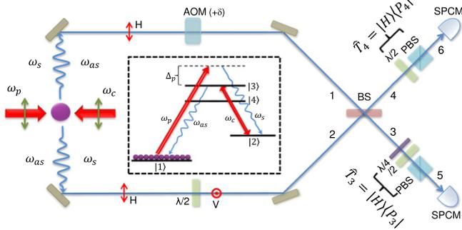
**Figure 1.** Schematic of experimental setup for producing narrow-band biphotons with frequency-bin entanglement. The phase-matched paired photons are generated from spontaneous four-wave mixing in laser-cooled  $^{85}\text{Rb}$  atoms with a right-angle pump-coupling geometry. The relevant  $^{85}\text{Rb}$  energy levels are  $|1\rangle = |5S_{1/2}, F = 2\rangle$ ,  $|2\rangle = |5S_{1/2}, F = 3\rangle$ ,  $|3\rangle = |5P_{3/2}, F = 3\rangle$ , and  $|4\rangle = |5P_{3/2}, F = 2\rangle$ .
