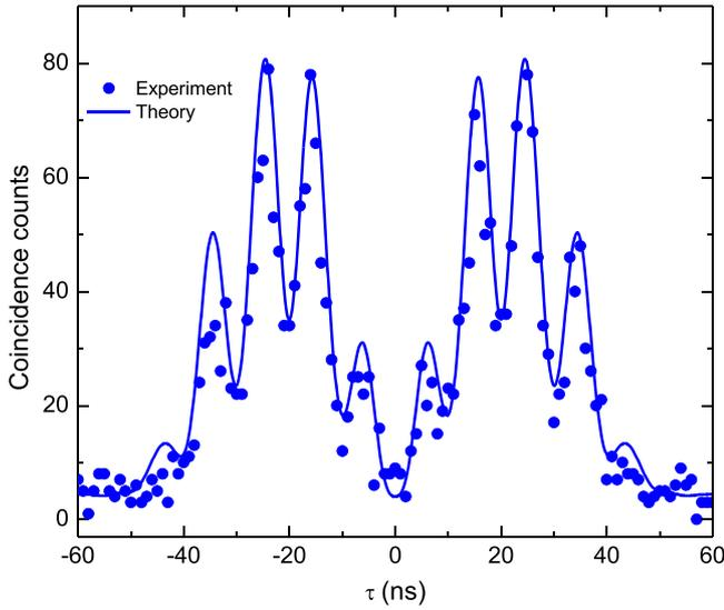
**Figure 4.** The two-photon beating with  $\phi = \pi/12$  and  $\theta = \pi$ . The experimental visibility is  $(51 \pm 5)\%$ .
