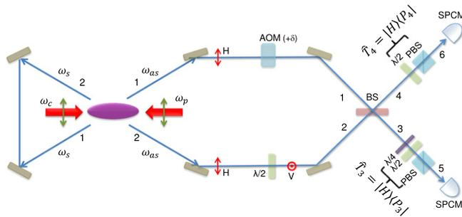
**Figure 5.** A possible experimental setup for generation of subnatural-linewidth frequency-bin entangled biphotons.
