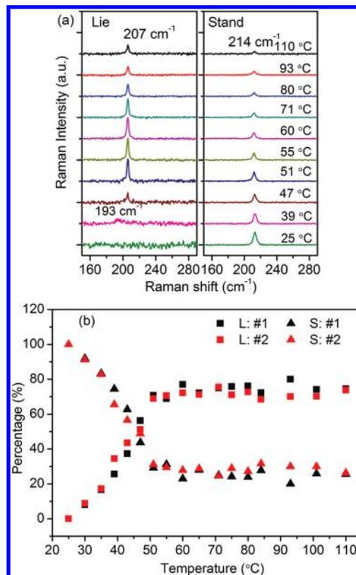
**Figure 4.** (a) Polarized Raman spectra of the low loaded  $I_2@AEL$  measured at different temperature with lying and standing configurations. (b) The percentage of lying (square) and standing (triangle) integrated Raman signals of the  $I_2@AEL$  at different temperature. #1 and #2 are the results of two independent samples.
