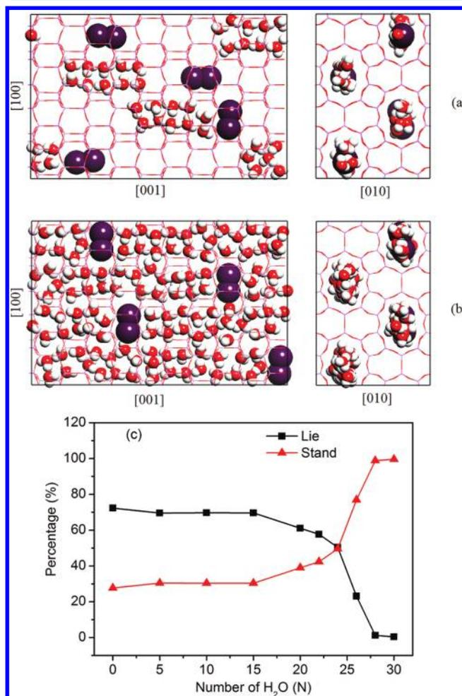
**Figure 3.** Snapshots of the MD simulations of low loaded  $\text{I}_2@AEL$  projected in (101) and (110) plane with 10 (a) and 30 (b) water molecules in each channel of simulation box. (c) MD simulation results of the percentage of lying (square) and standing (triangle) iodine molecules as a function of the loading of water molecules.
