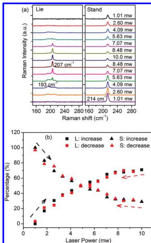
**Figure 6.** (a) Polarized Raman spectra of low loaded  $I_2@AEL$  measured at different laser power with the lying and standing configurations. The laser power increases from 1.01 to 10 mW and then reverses back. (b) The percentage of lying (square) and standing (triangle) integrated Raman signals of the  $I_2@AEL$  with increase and decrease of laser power. The arrows represent the sequence of the data in the same color.
