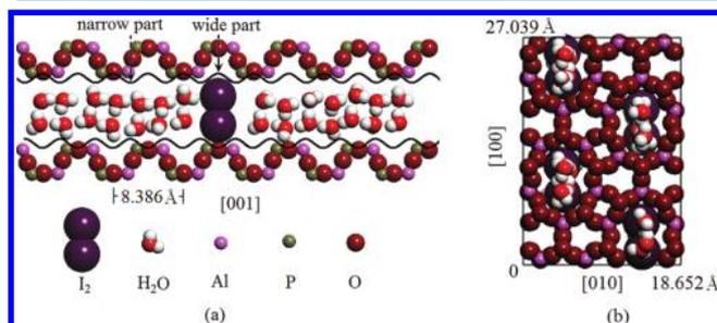
**Figure 1.** (a) Schematic view of the hydrated AEL channels with low loading iodine molecules. The potential energy described by the quasi-sinusoidal lines at the end of the major axes of the ellipses shows that the channel changes between wide part and narrow part with a period of  $1/2 c$ , where  $c = 8.386 \text{ \AA}$  is the lattice constant in the channel axis of the AEL crystal. (b) The low loaded  $\text{I}_2$ @AEL projected in the (110) plane with periodic conditions.
