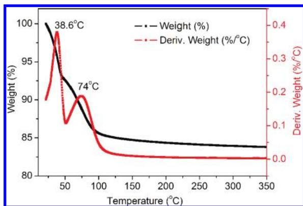
**Figure 5.** Thermal gravimetric curve and the corresponding derivative curve of high loaded  $I_2@AEL$ . The two features of the derivative curve correspond to desorption of water molecules (38.6 °C) and iodine molecules (74 °C).
