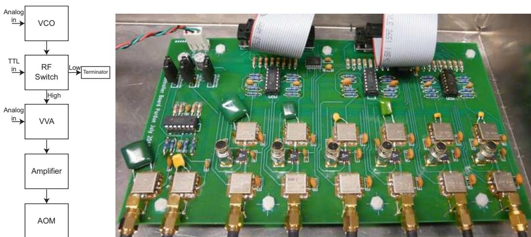
Figure 3.7. The board used to control the AOMs in our setup (right) can be thought of as a series of channels (left) with a VCO, RF Switch, VVA on the board, with a high power amplifier driving an AOM after the board. The devices can be controlled by outputs coming from a data acquisition system programmed by a computer.
