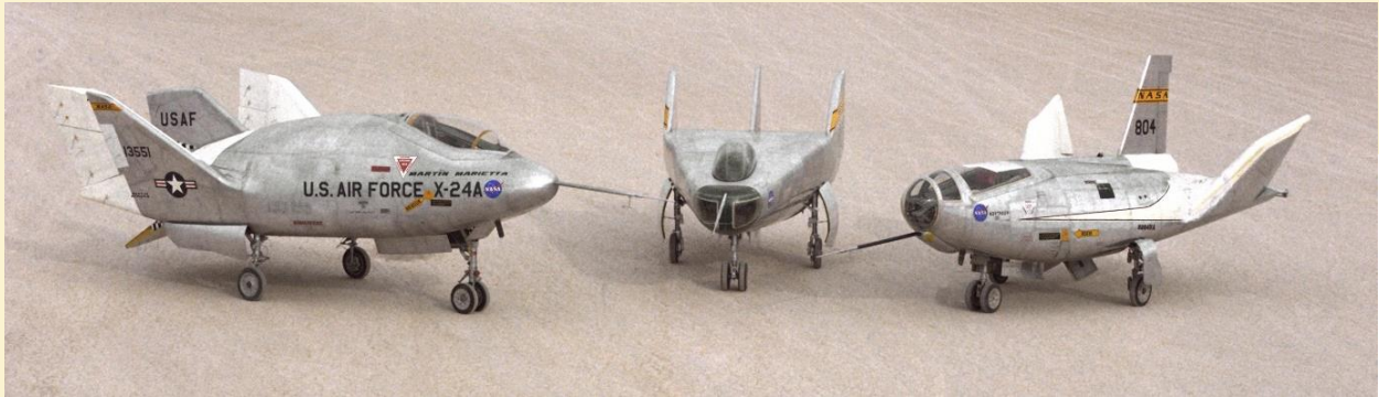
Figure 1: Lifting body designs (left-right) X-24, M2-F3, and HL-10 (photo: NASA)
