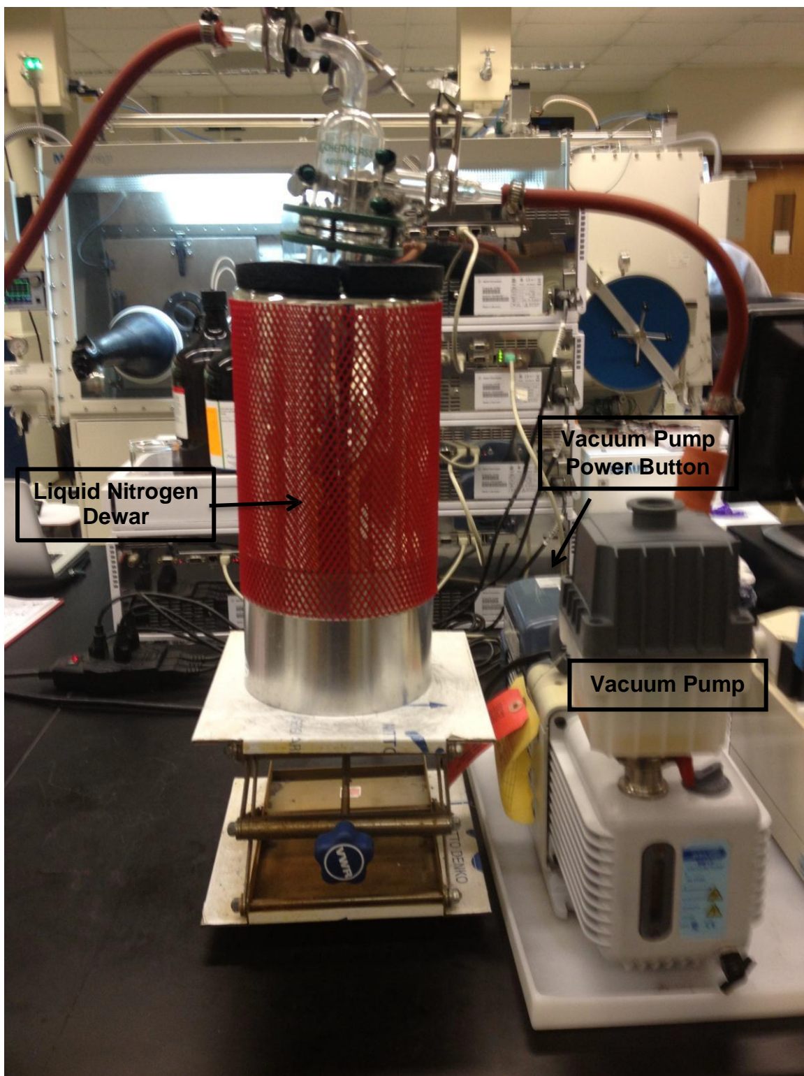
Figure A2. Liquid nitrogen dewar, vacuum pump, and power button located behind the pump.
