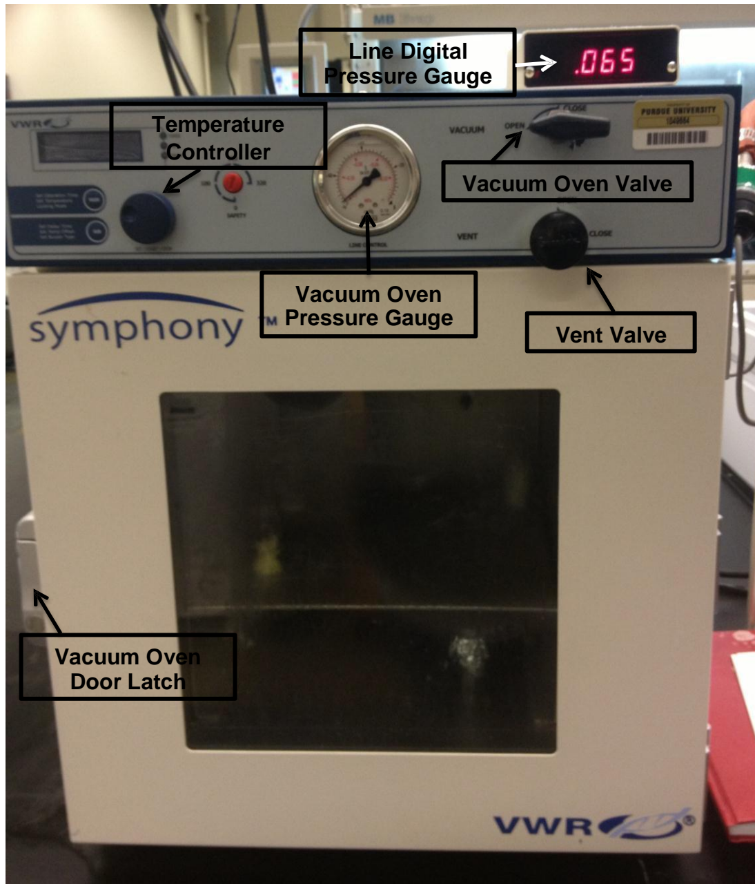
Figure A1. Vacuum oven, temperature controller, vacuum oven door latch, vacuum oven pressure gauge, line digital pressure gauge, vent valve, and vacuum oven valve.
