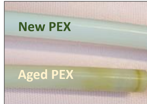
One year old PEX pipe pulled from the ReNEWW House
