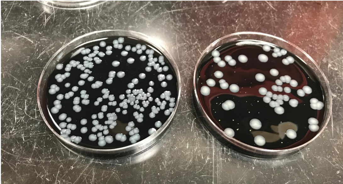
The detection of Legionella species in water samples using cell culture. Left, water sample AS (After softener); right, water sample HWRa (Hot water recirculation).
