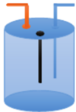
Side-feed water heater A variant configuration. This variation and variation in dip tube length and shape in traditional heaters present challenges to general water heater models.
