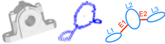
Figure 2 (a) 3D model, (b) Skeleton, and (c) Skeletal graph for a bearing block. L represents loop entity while E represents line entity in the skeletal graph
