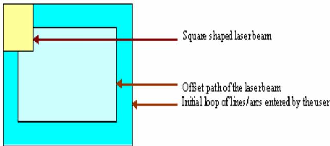
Figure 12: Through-cut machining path
