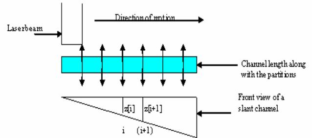
Figure 14: Machining path for a tapered channel
