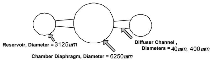
Figure 19: Schematic of Micropump
