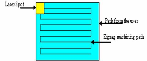
Figure 13: Zigzag laser machining path for a Pocket feature
