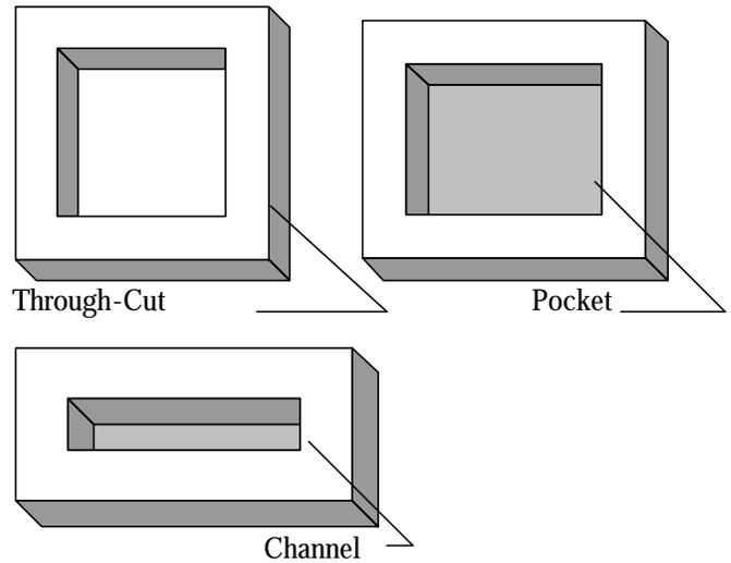
Figure 3: Laser based micro-machining features
