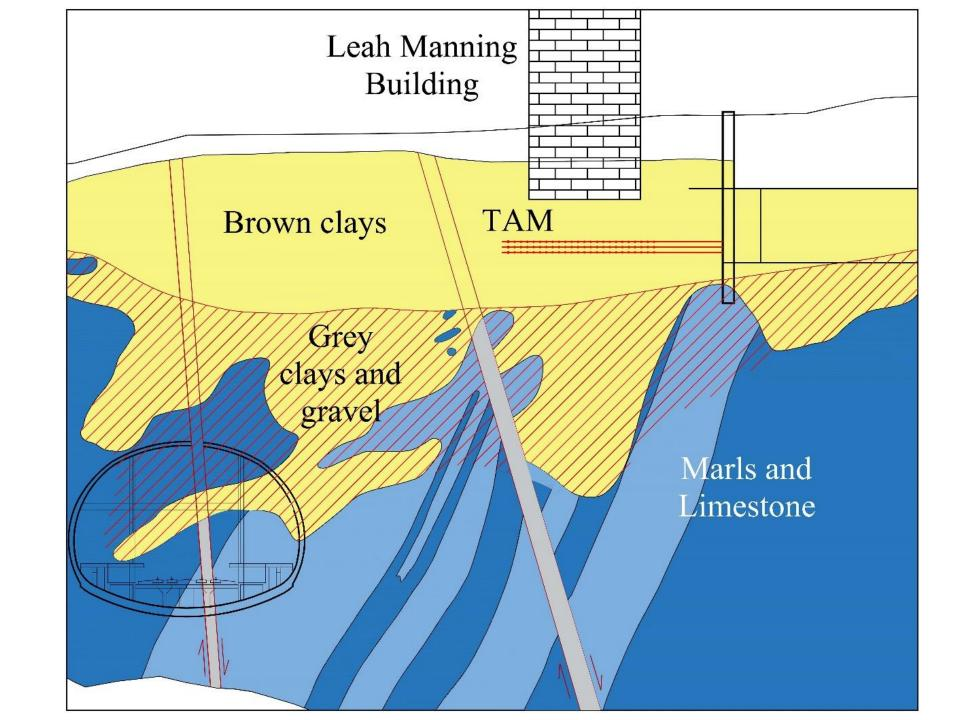
Ground water lowering induced by tunnel construction and building settlement
