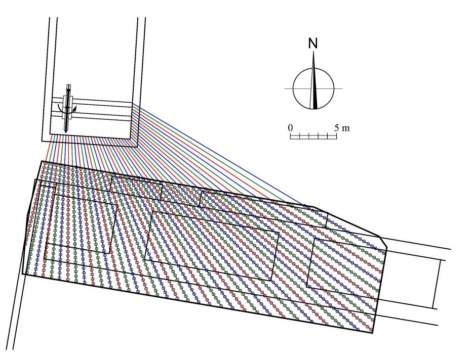
Three levels of compensation grouting boreholes
