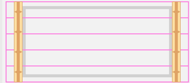
B. Install Geotextile over Lagoon and Place Stabilizing Berm
