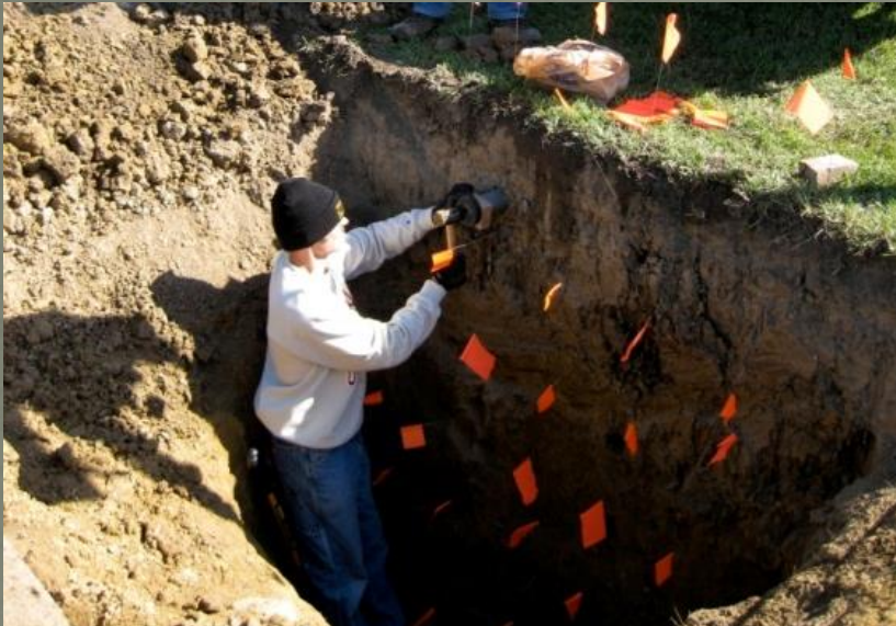
Extensive core sampling for analysis of physical and thermal properties
