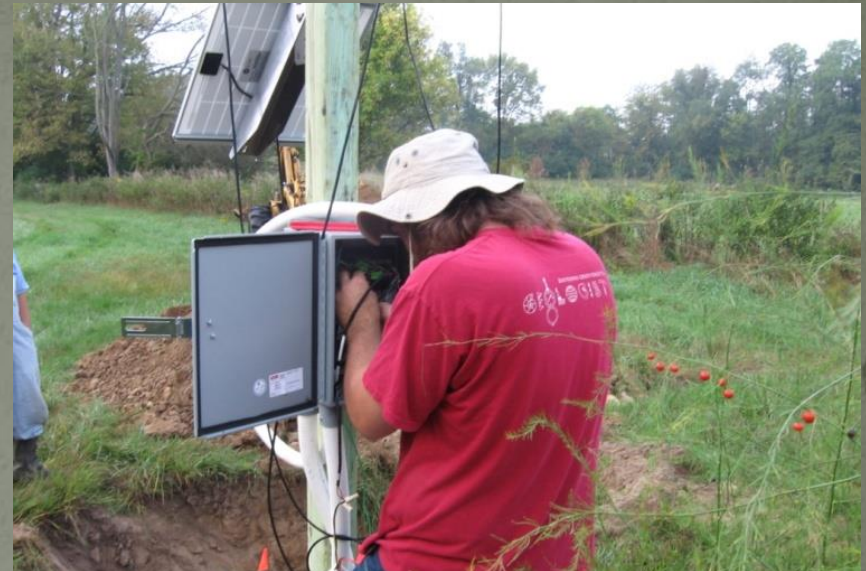
Automated data logging and cellular telemetry for real-time data acquisition
