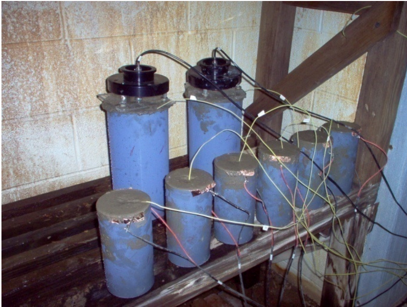
Finished specimen with sensors
