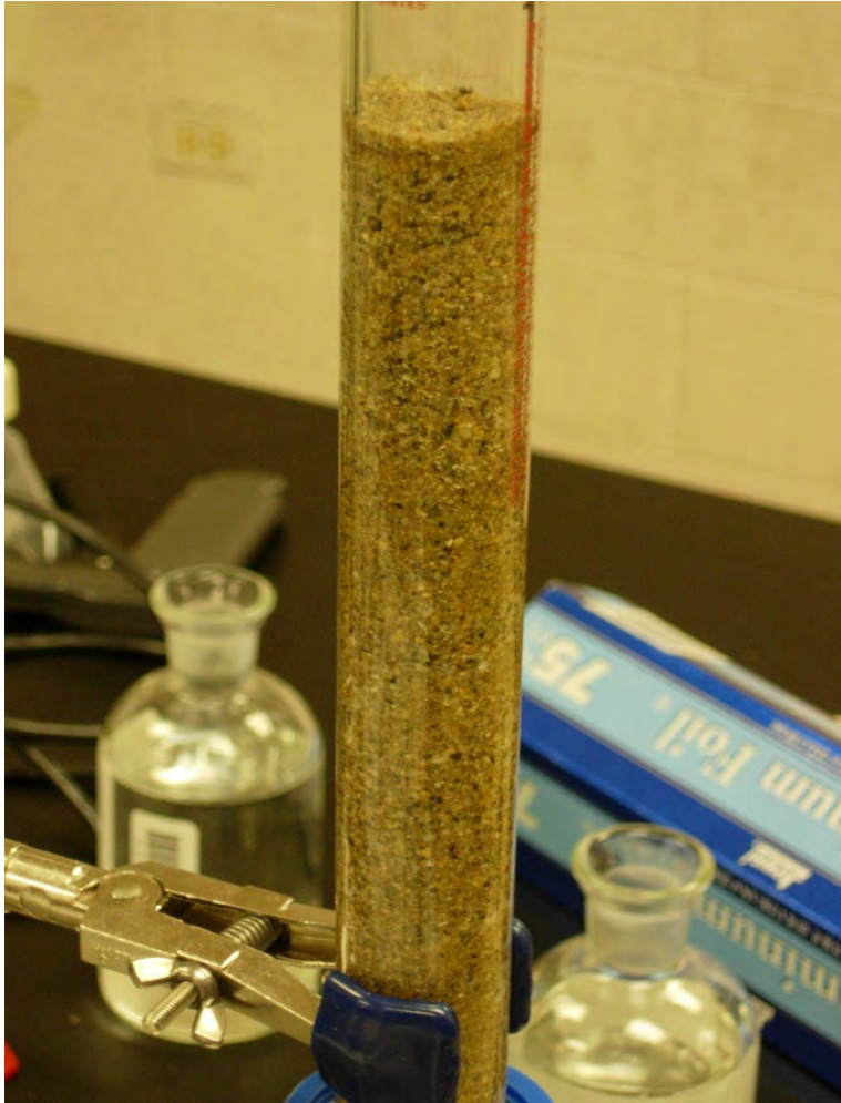
Bare NIP stack at the top of the soil column after about 20 pore volume of flushing under 30psi
