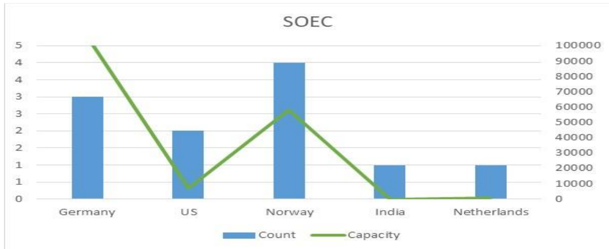
Figure 8 SOEC electrolyser upcoming capacities 5
