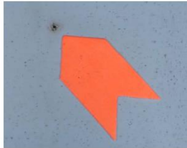
Pinhole failure of separator
