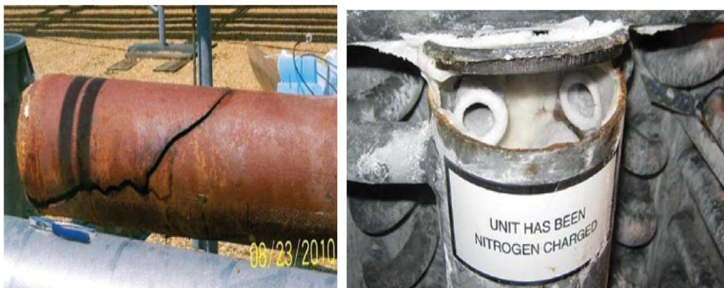
Figure 1. Ruptured low temperature suction line (left), Evaporator coil weld failure (right) [4]
