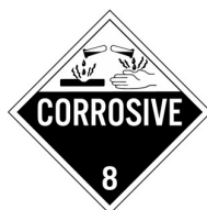
Figure 3. Hazardous materials warning label for Sulfuric acid transportation
