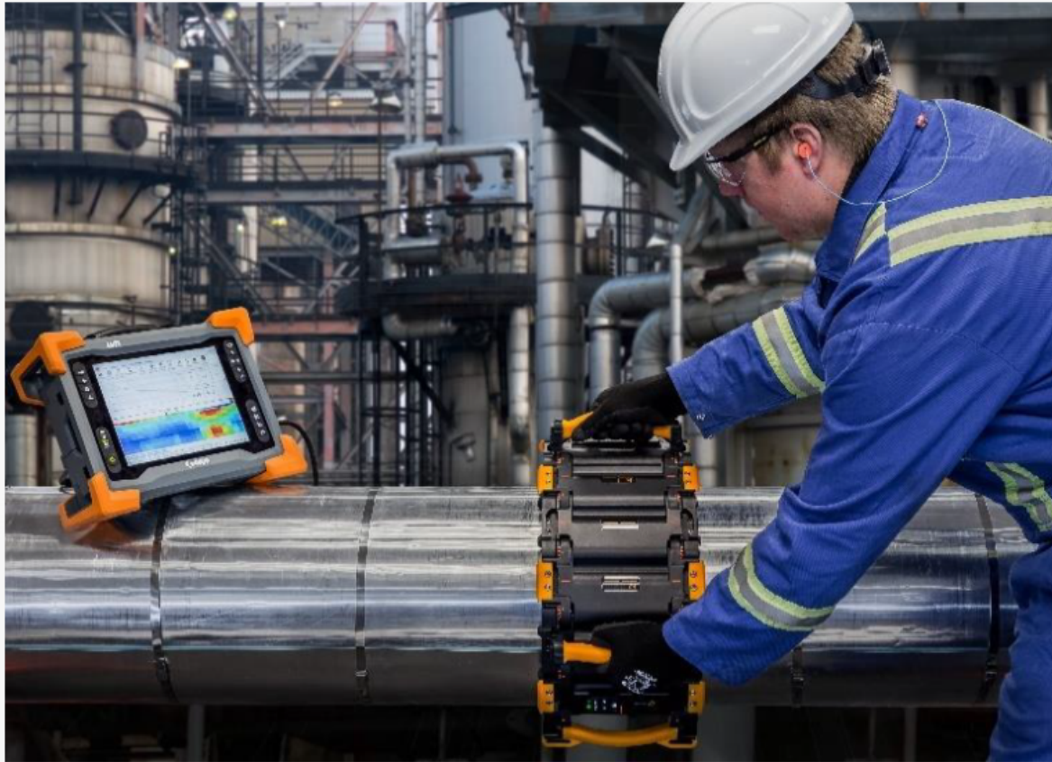
Figure 8. How pulsed eddy current technique is used in the plant. 12
