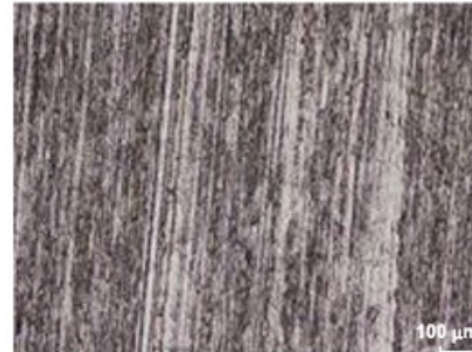
Entry 6. Lot B Corrosive Mass loss = 7.6 mg 37 mil/yr
