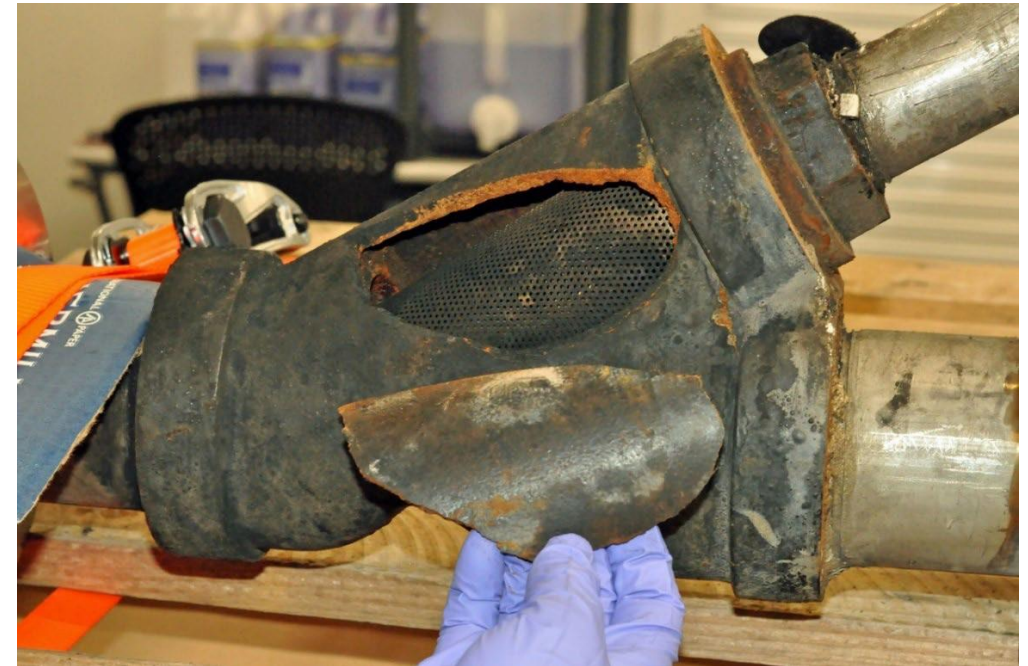
Figure 18. Y-Strainer Piece. This photo shows the single piece that broke away from the failed y-strainer. (Credit: CSB)
