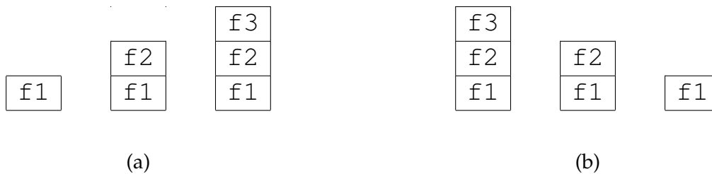
Figure 2.2: (a) The stack changes after f_1 , f_2 , and f_3 are called. Each function call pushes the called function onto the stack. (b) When f_3 finishes, it is popped from the stack and now f_2 is at the top. When f_2 finishes, it is popped from the stack and f_1 is at the top.
