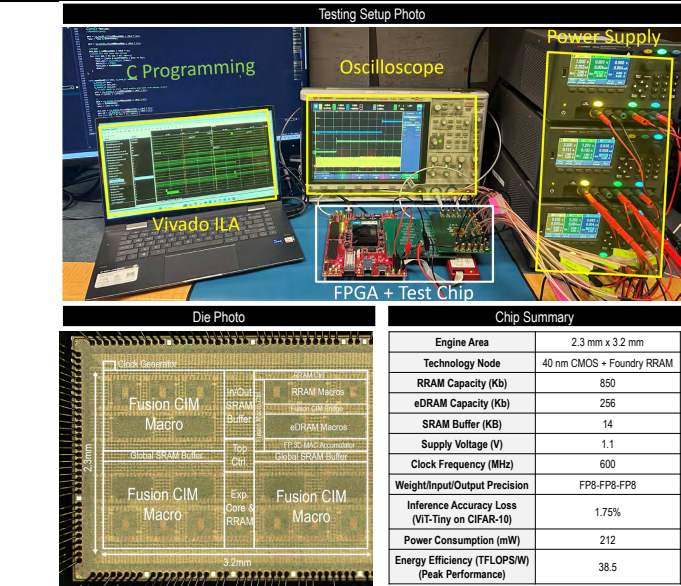
Fig. 7. CENTAUR’s testing setup, die photo and chip summary.
